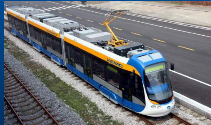
公司新研制的100%低地板新型城市有轨电车 XEMC newly developed 100% low floor light rail vehicle .
