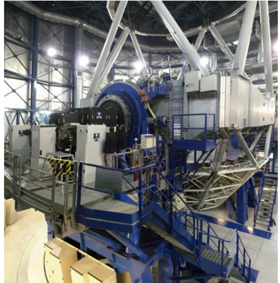
Multi-conjugate adaptive optics demonstrator (MAD) installed on Nasmyth A of UT3
